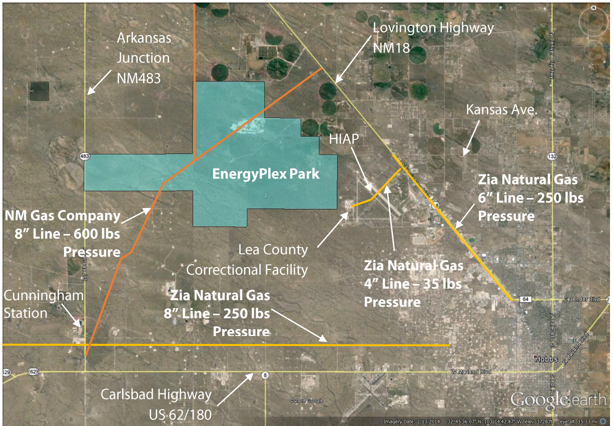
Figure 12: Existing natural gas lines
