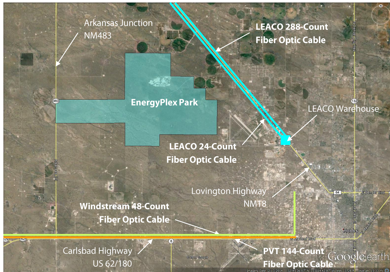
Figure 11: Existing fiber optic cables
